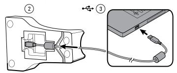
Place the RetinaVue 100 Imager on the docking station charger with the contact pins of the RetinaVue 100 Imager touching the contact pins of the docking station charger.
