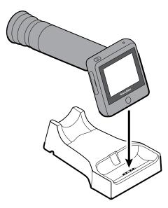
5. Before the first use, allow the RetinaVue 100 Imager to charge for 8 hours on the docking station charger.
