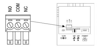
Connect the wires from the signaling device to the screw terminals. Plug the terminal connector into the socket on the clock. Only one (1) wire should be inserted into the terminal block positions NO and COM, all wire splices should be done externally. See the following diagrams for details.
