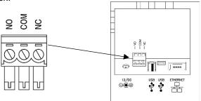
Connect the wires from the door access device to the screw terminals. Plug the terminal connector into the socket on the CT clock. Only one (1) wire should be inserted into the terminal block positions NO and COM, all wire splices should be done externally. See the following diagrams for details.
