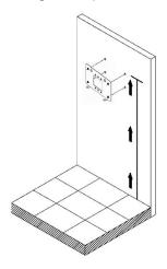
Note: The bottom of the clock should be about **45** inches from the floor.
