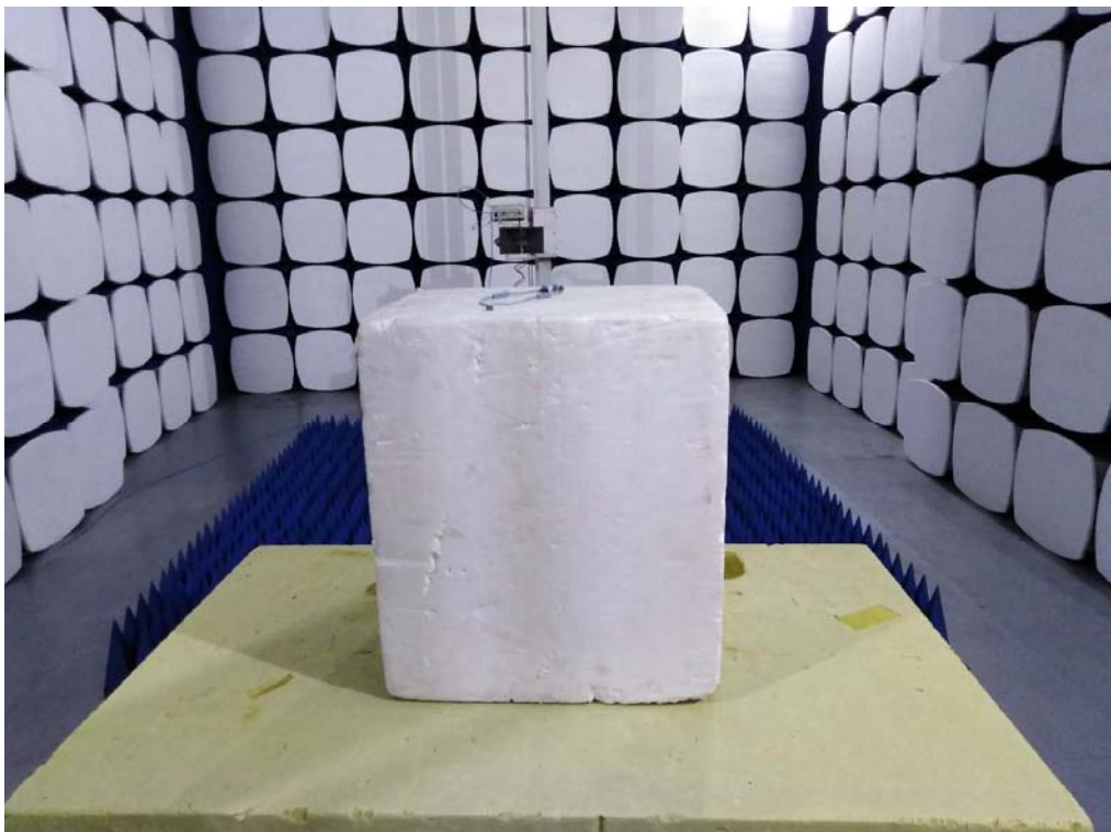
Radiated Setup photo (Above 1G)
