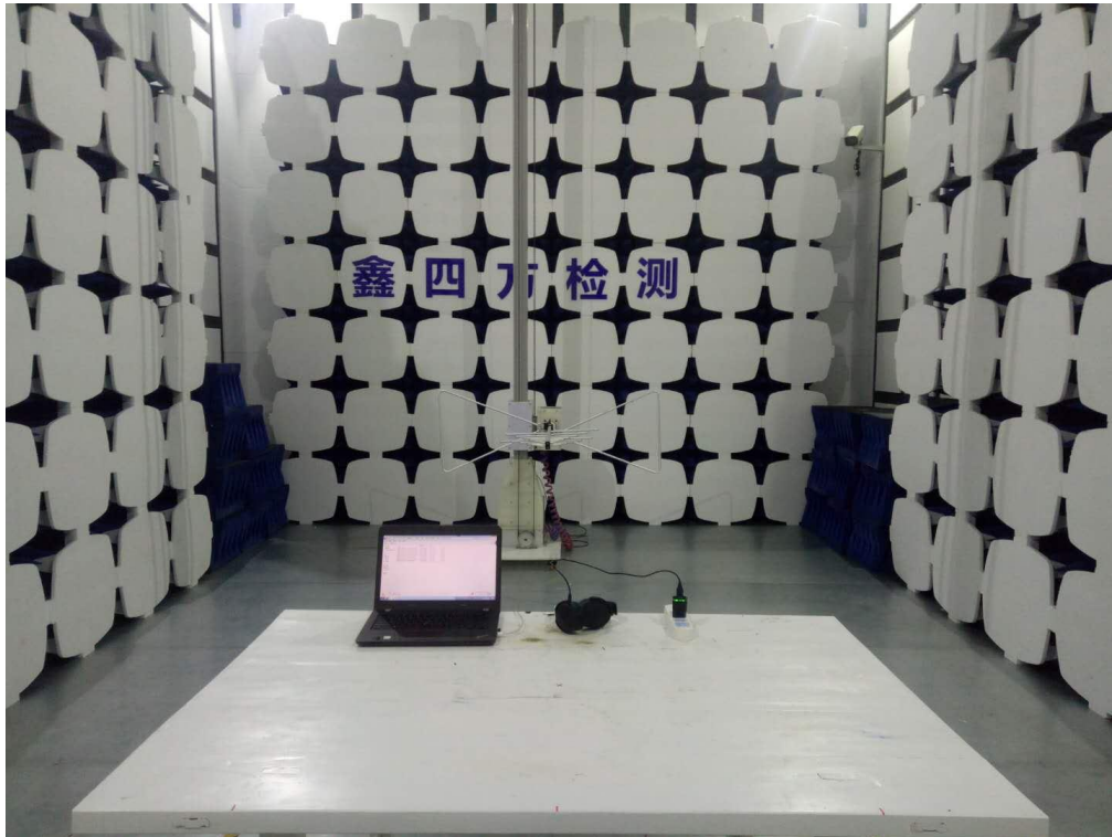
radiated emission test 30MHz – 1GHz
