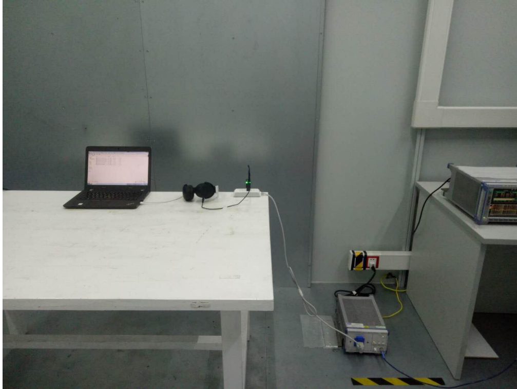
radiated emission test 30MHz – 1GHz
