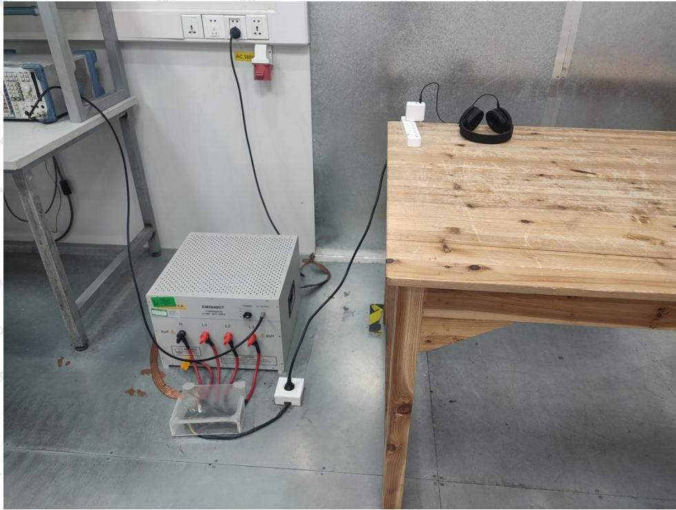
Photo of Conducted Emission Measurement
