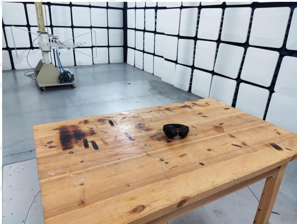
Photo of Radiation Emission Test
