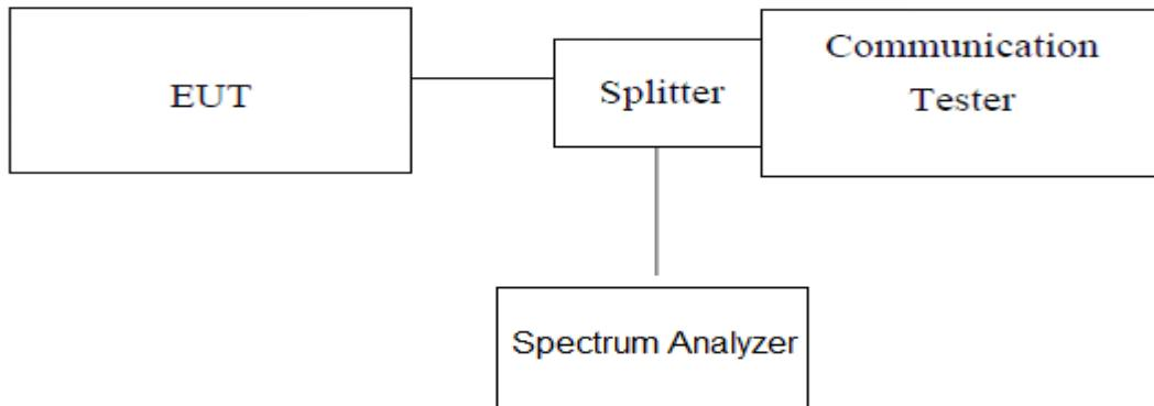
*Note: Measurement setup for testing on Antenna connector*
