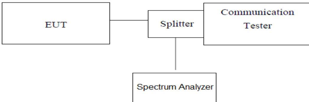
*Note: Measurement setup for testing on Antenna connector*
