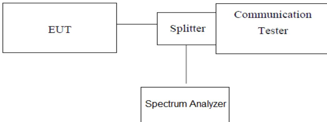
*Note: Measurement setup for testing on Antenna connector*
