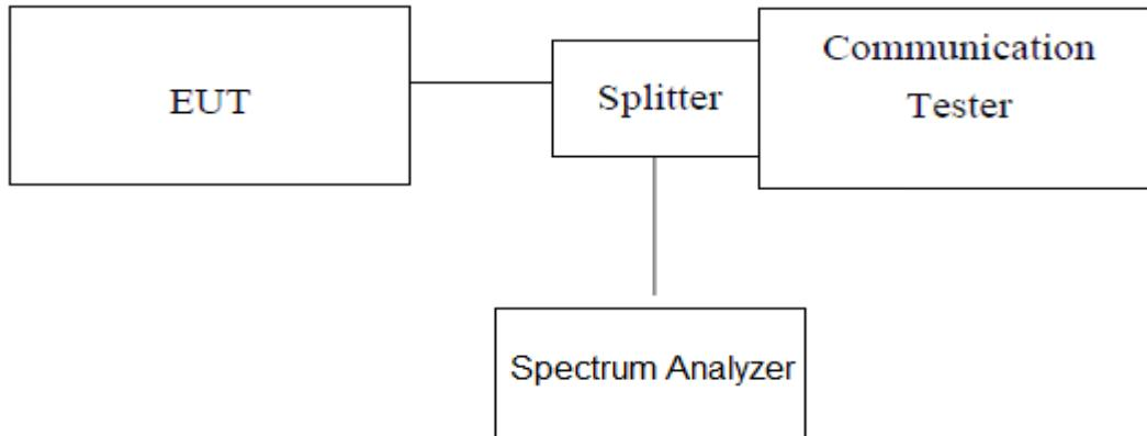
*Note: Measurement setup for testing on Antenna connector*
