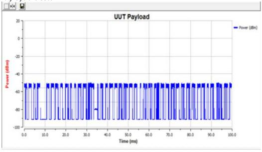
The EUT was configured to communicate with a client device. The MPEG test file was streamed from the Master (EUT) to the Client on the selected test channel. Channel move was disabled. Measurements were made while utilizing all the bandwidths of the EUT.
