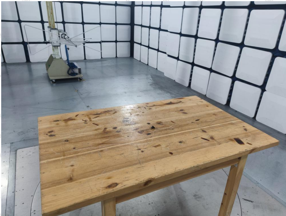
Photo of Radiation Emission Test
