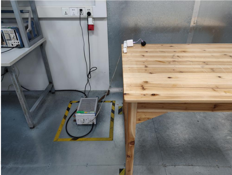
Photo of Conducted Emission Measurement
