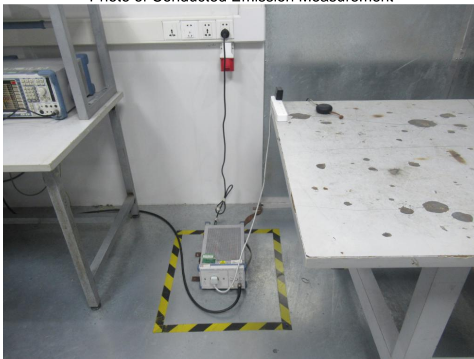
FCC ID: 2AF9P-FEM Photo of Conducted Emission Measurement
