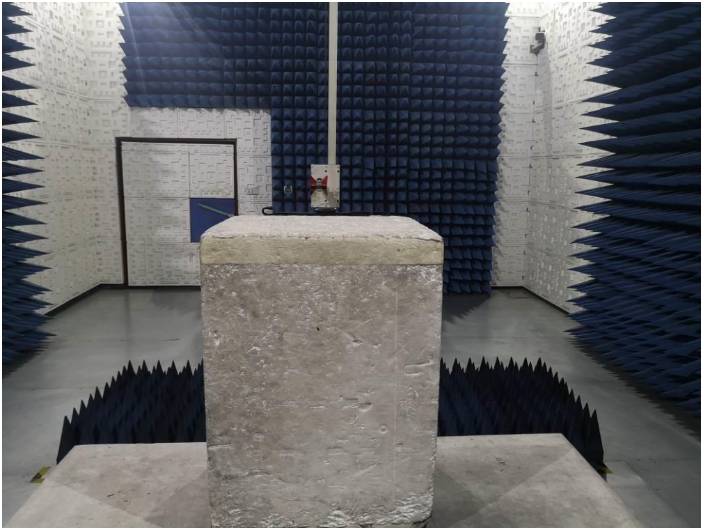
RADIATED EMISSION TEST SETUP ABOVE 1GHZ
