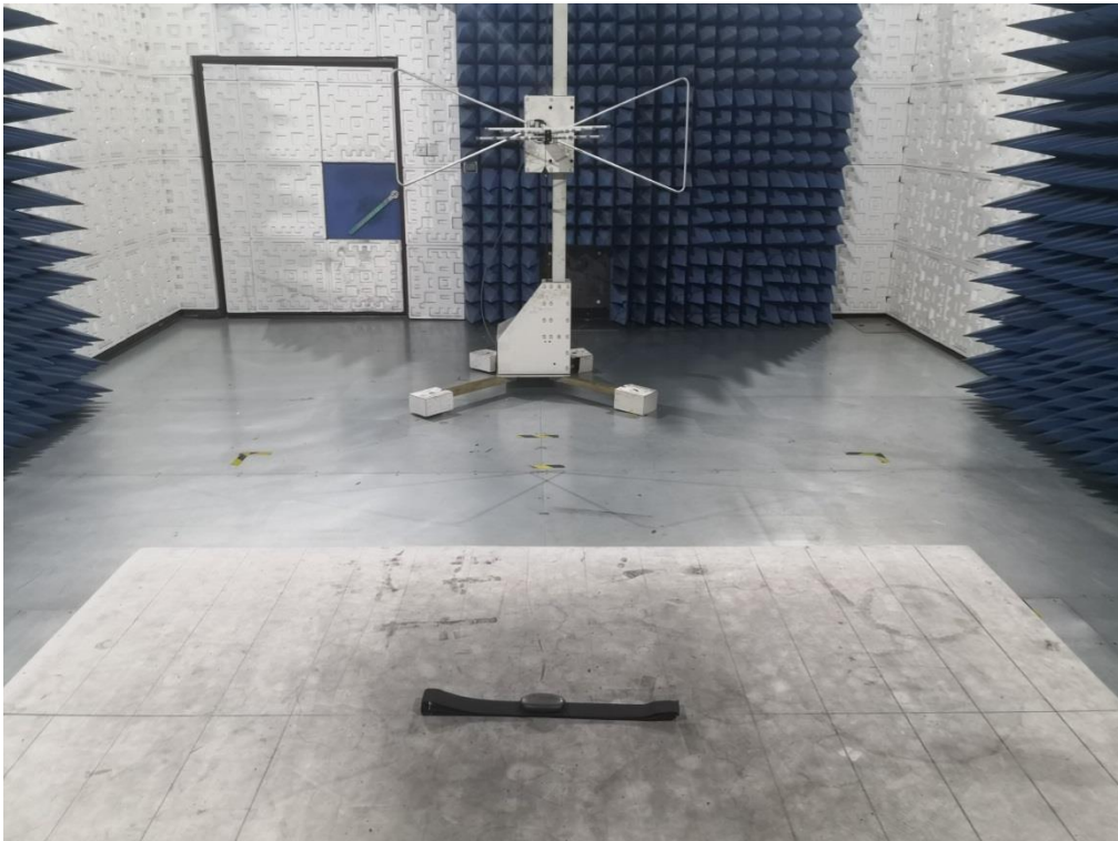
RADIATED EMISSION TEST SETUP ABOVE 1GHZ
