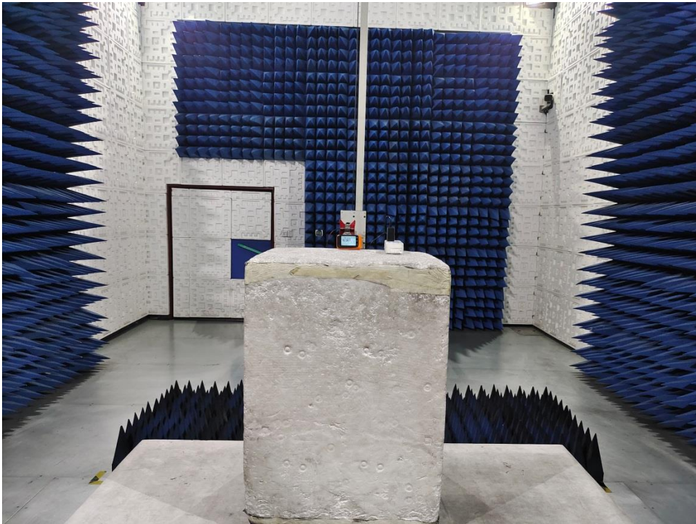
RADIATED EMISSION TEST SETUP ABOVE 1GHZ
