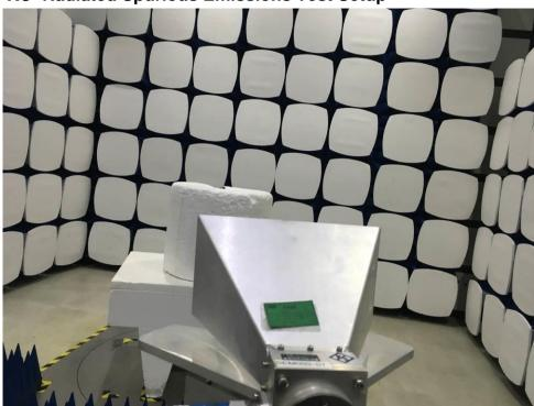
**1.3** Radiated Spurious Emissions Test Setup
