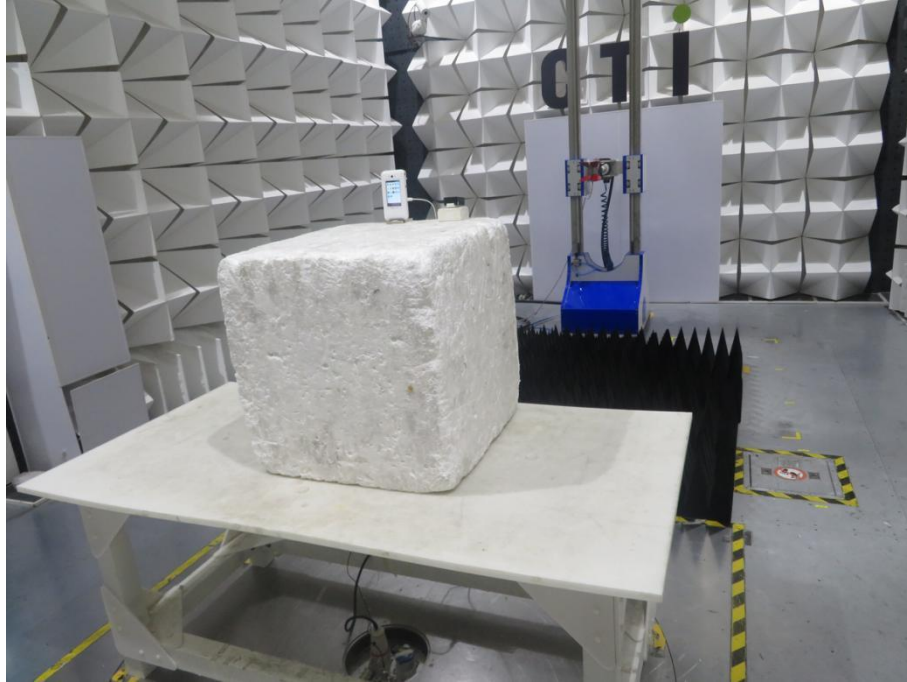
Radiated spurious emission Test Setup-2(Above 1GHz)
