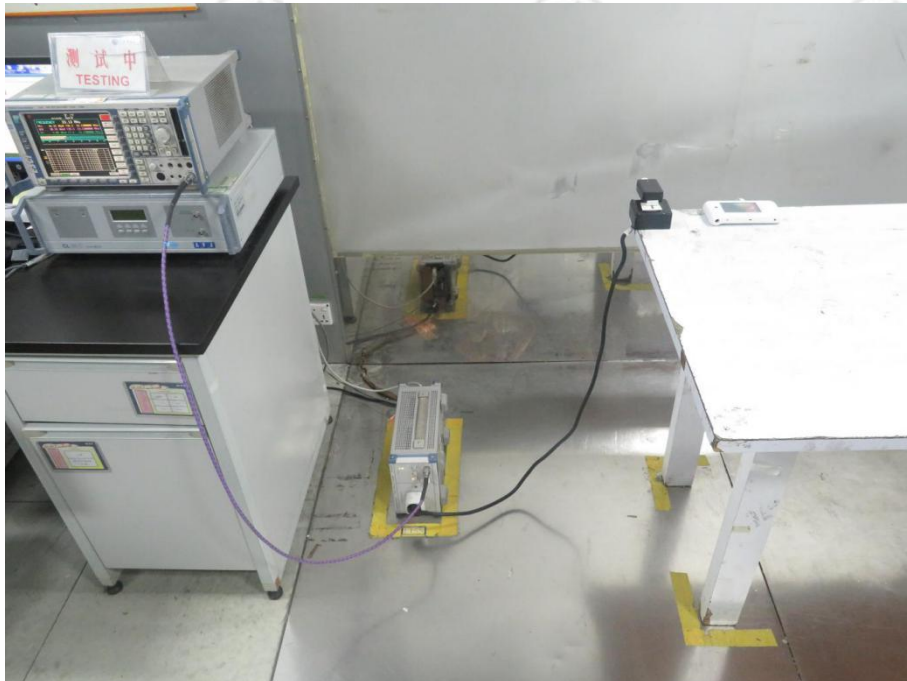
Conducted Emissions Test Setup
