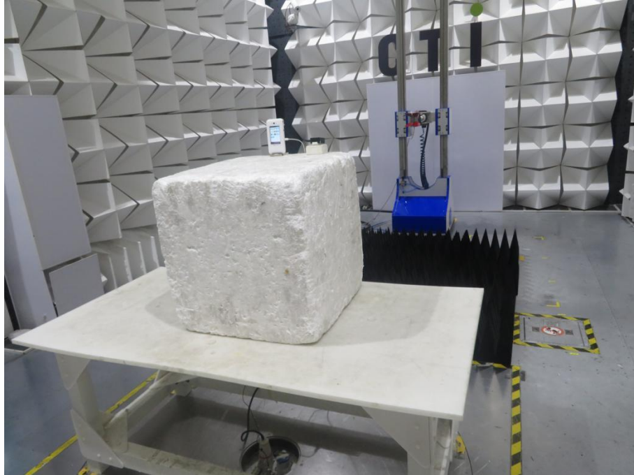
Radiated spurious emission Test Setup-3(Above 1GHz)
