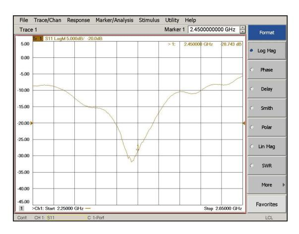
Impedance and Return Loss Test-Body(2017.2.10)
