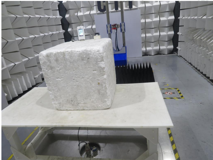
Radiated spurious emission Test Setup-2(Above 1GHz)
