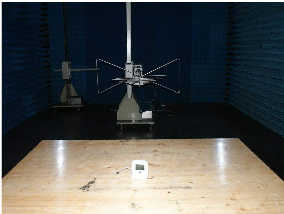
Photograph 4: Set-up for Radiated Spurious Emission, 30MHz - 1GHz
