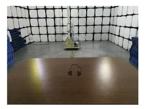
Radiation Emission Test Setup (1GHz to 18GHz)
