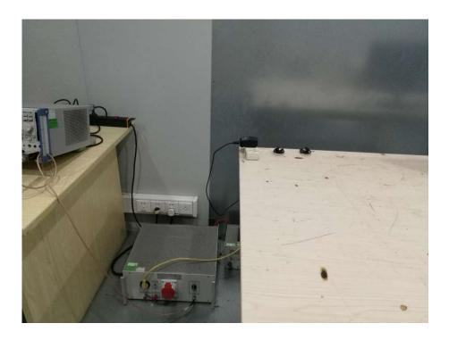
Radiation Emission Test Setup (Below 30MHz)
