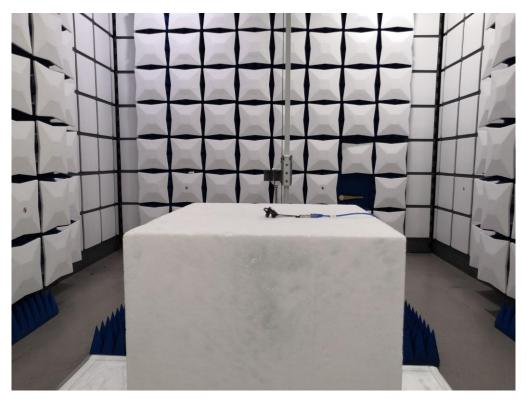
**Left**FCC RADIATED EMISSION TEST SETUP
