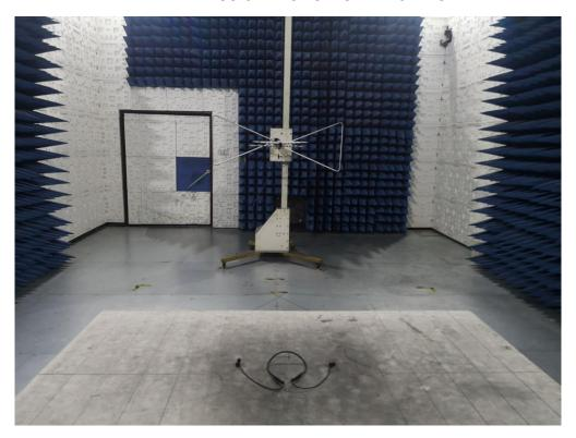
RADIATED EMISSION TEST SETUP ABOVE 1GHz
