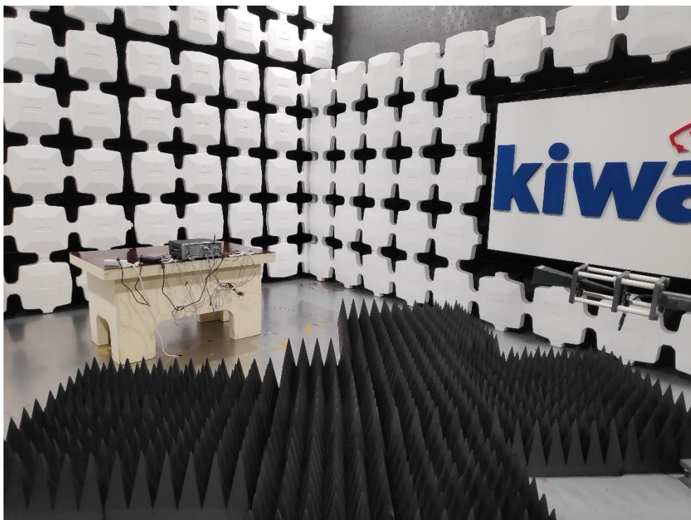
Photo 4 Photograph test setup radiated emissions 18 – 26.5 GHz, report section 3.1
