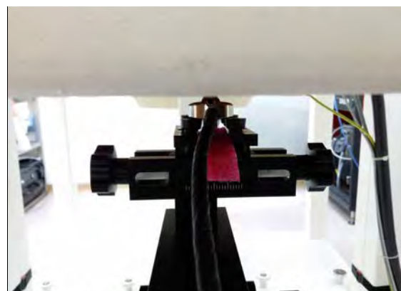
Fig.4 EUT Back side to flat phantom
