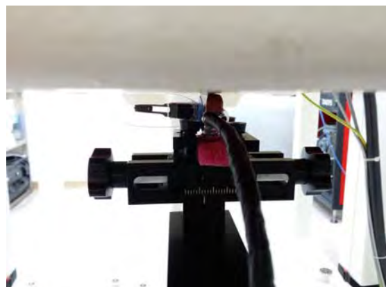
Fig.5 EUT Top side to flat phantom
