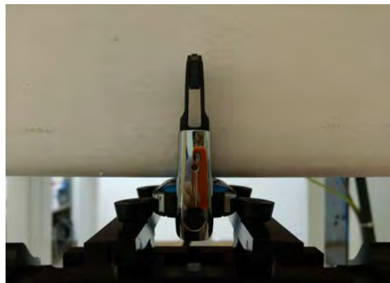
Fig.3 EUT Front side to flat phantom
