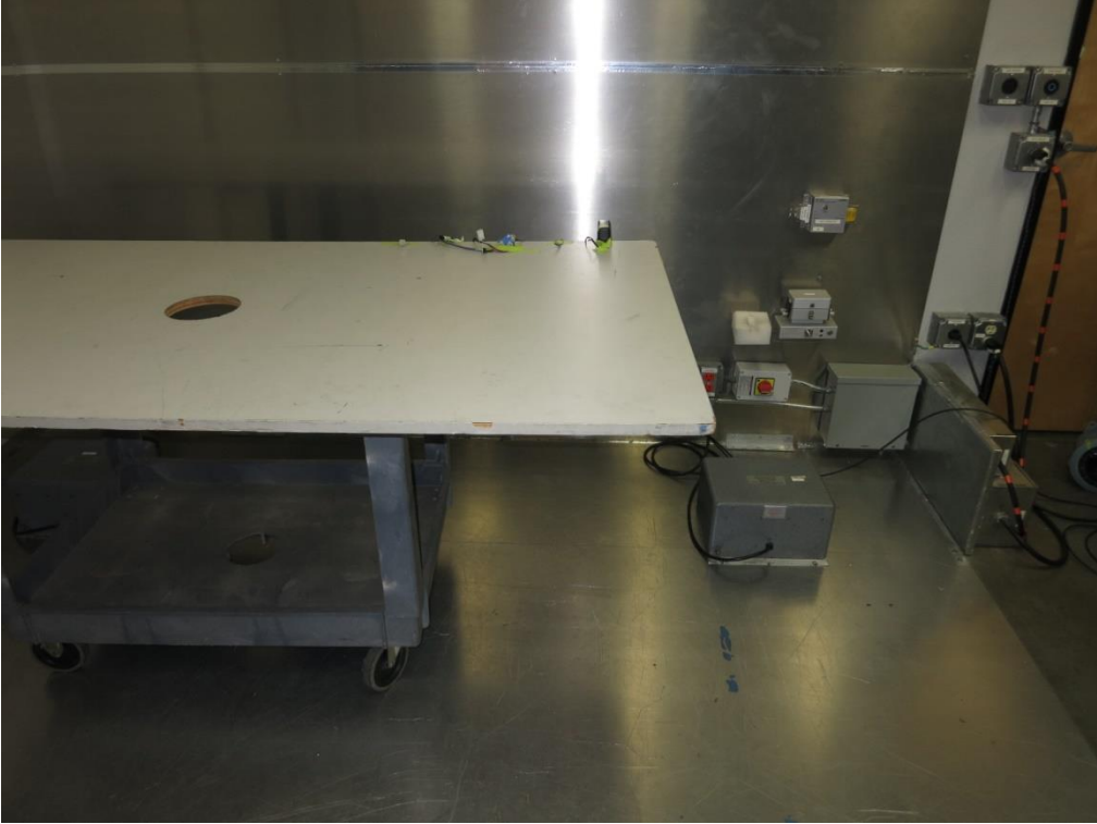
Power Line Conducted Emissions
