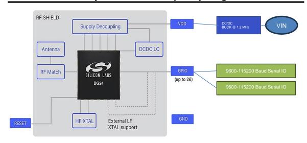
HF XTAL = 39.000 MHz +/-42 ppm max over temperature and setpoint
