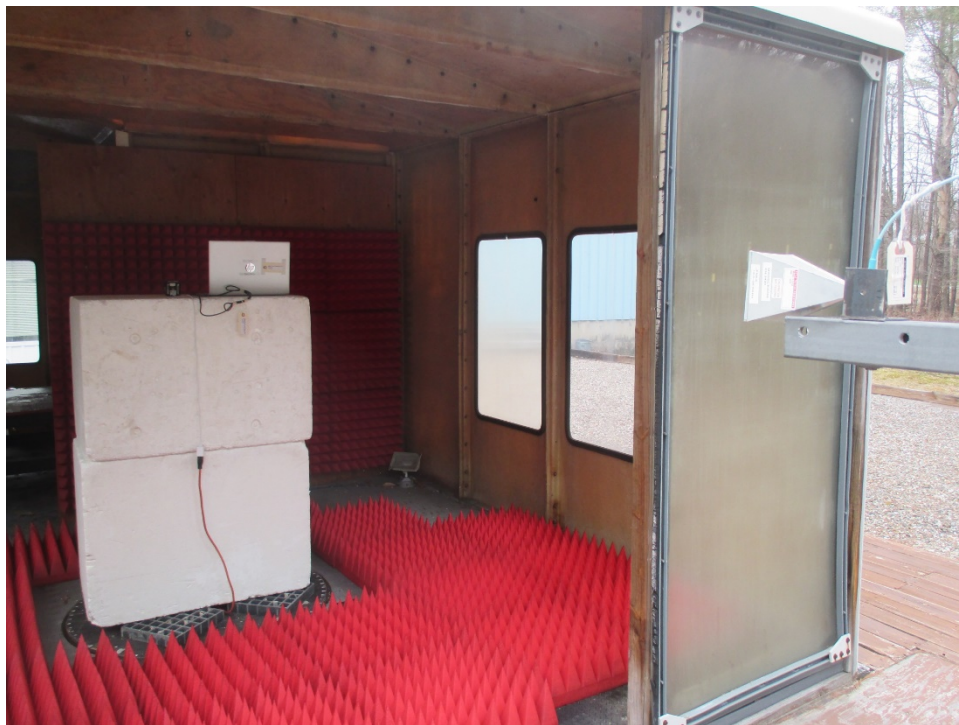
Vertical Polarization, 18 to 26 GHz
