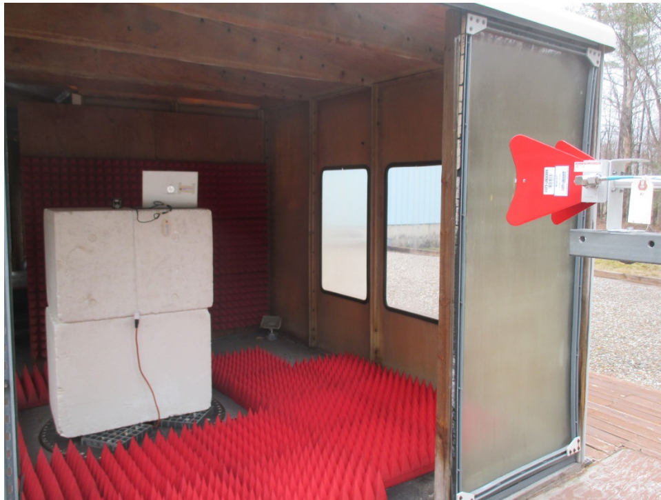
Horizontal Antenna Polarization, 1 to 18 GHz
