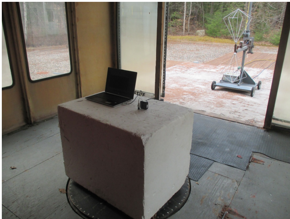
Vertical Antenna Polarization, 30 to 200 MHz
