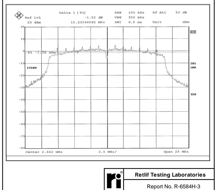
FCC Part 15, Subpart C, Section 15.247(b)(3) Conducted Emissions, Power Output Test Data
