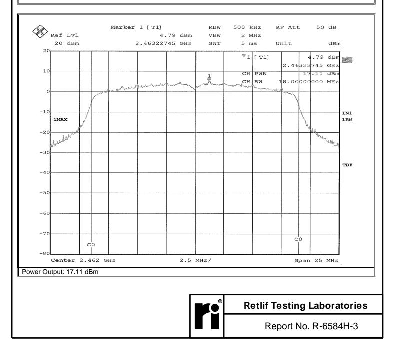
FCC Part 15, Subpart C, Section 15.247(d) Antenna Port, Conducted Emissions Band Edge Test Data
