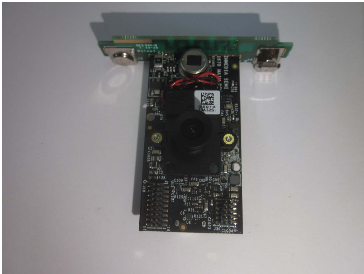
Main Board, Battery /LFR Antenna Board Attached, Side 2 Battery /LFR Antenna Board bottom
