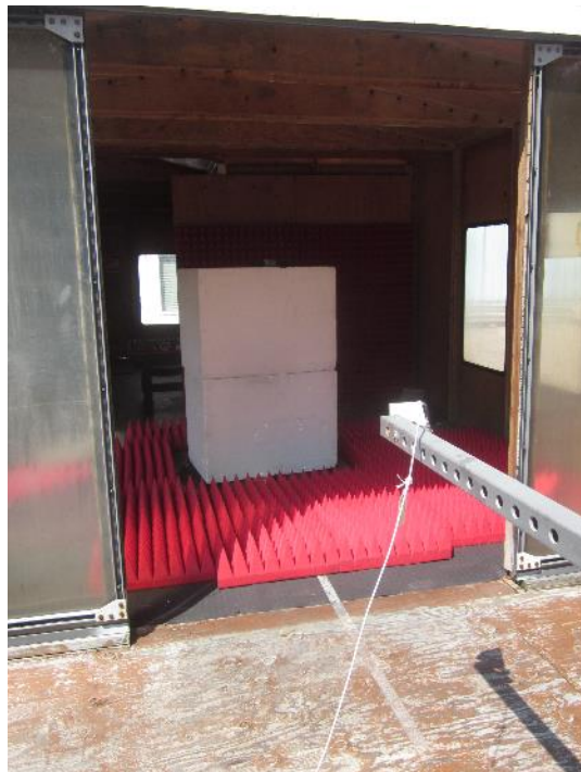
Vertical Polarization, 18 to 25 GHz, High Gain Horn, 150 cm
