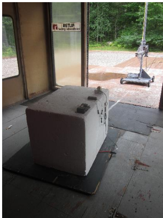
Vertical Polarization, 200 MHz to 1 GHz, Log Periodic, 80 cm
