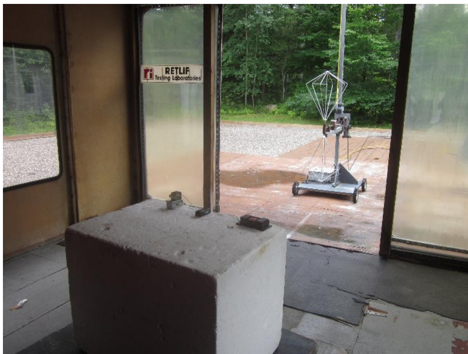
Vertical Polarization, 30 to 200 MHz, Biconical Antenna, 80 cm
