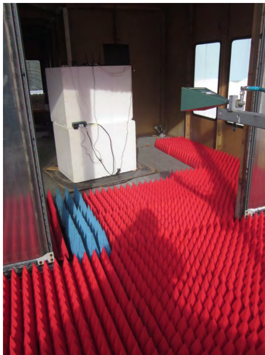
Vertical Polarization, 12- 18 GHz, High Gain Horn, 150 cm
