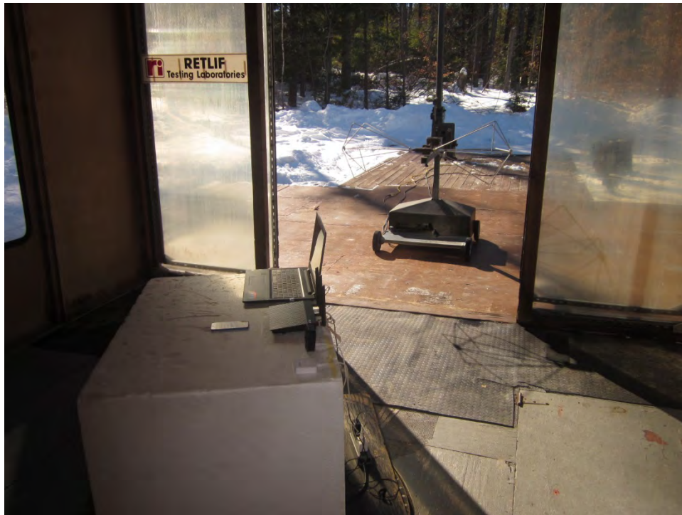
Horizontal Polarization, 30 MHz – 200 MHz, Biconical Antenna, 80 cm
