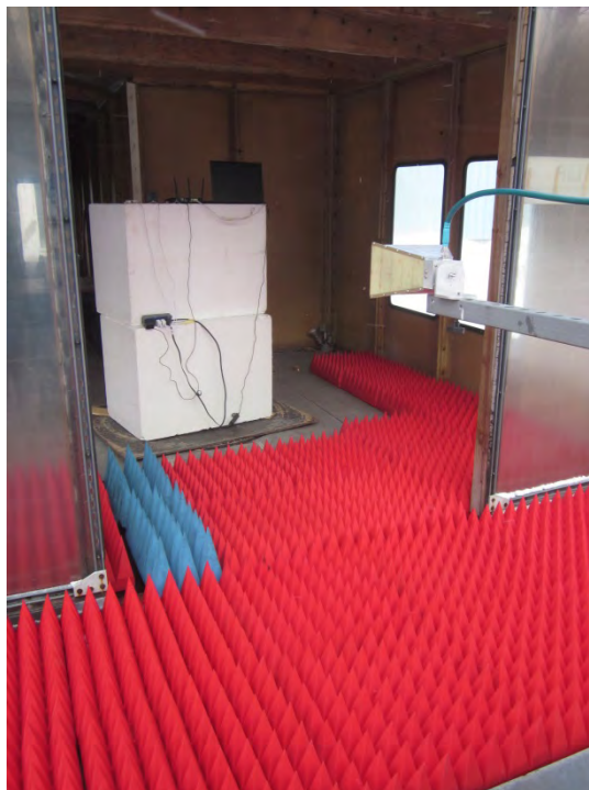
Vertical Polarization, 1- 12 GHz, Double Ridge Guide, 150 cm
