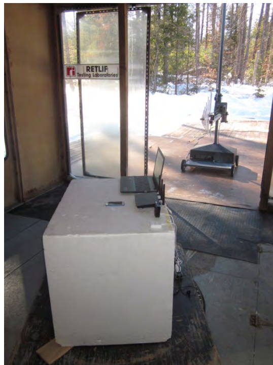
Vertical Polarization, 200 MHz - 1 GHz, Log Periodic, 80 cm
