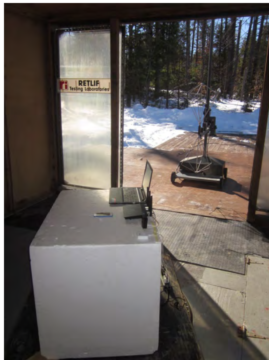
Vertical Polarization, 30 MHz – 200 MHz, Biconical Antenna, 80 cm
