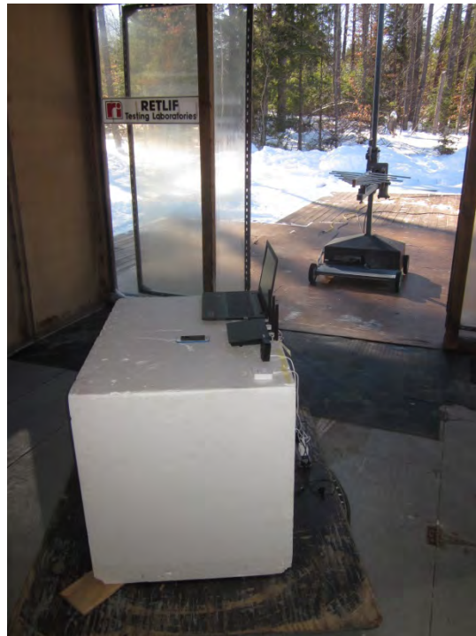
Horizontal Polarization, 200 MHz - 1 GHz, Log Periodic, 80 cm
