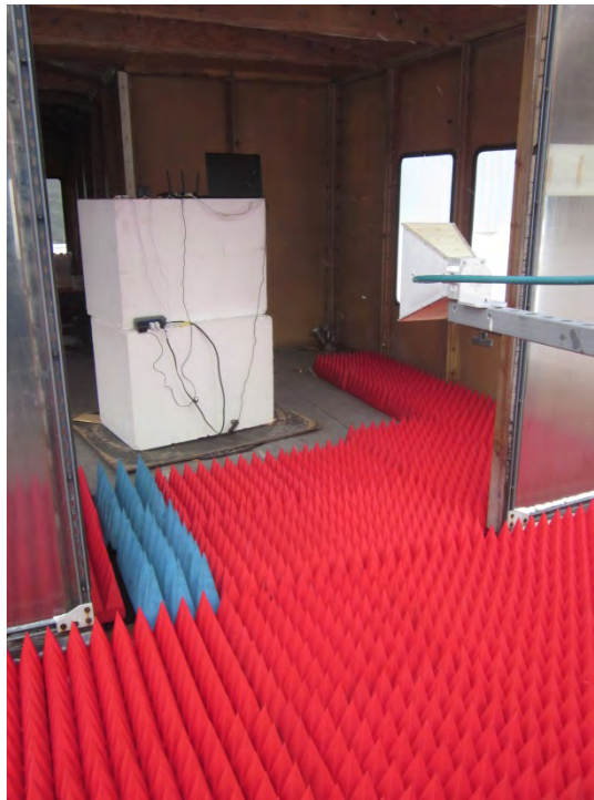
Horizontal Polarization, 1- 12 GHz, Double Ridge Guide, 150 cm
