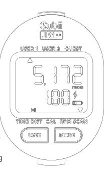
Press the MODE button to switch which metric is displayed. You can use the SCAN mode to automatically toggle between the above metrics every 7 seconds. The triangle indicator shows which view is selected.
