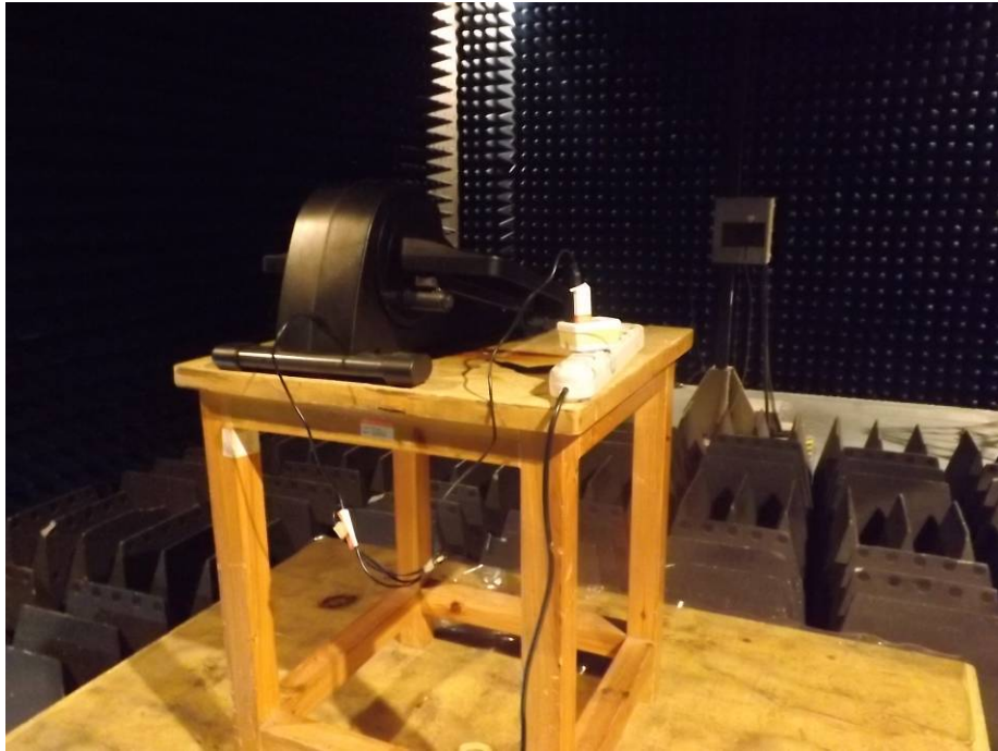
Photograph – Conducted Emission Test Setup at Test Site 1#
