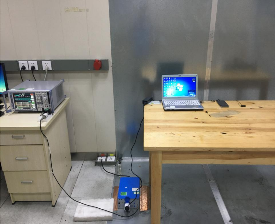
FCC RADIATED EMISSION TEST SETUP
