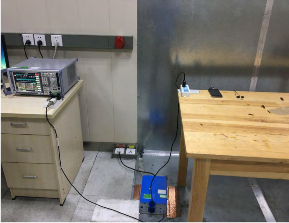
FCC RADIATED EMISSION TEST SETUP
