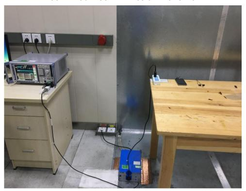
FCC RADIATED EMISSION TEST SETUP
