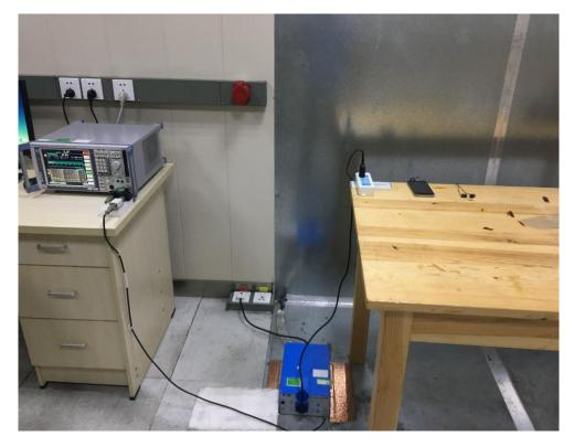
FCC RADIATED EMISSION TEST SETUP
