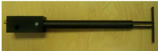
Figure 1 – MVG COMOSAR Validation Dipole
