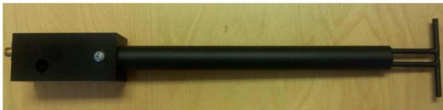
Figure 1 – MVG COMOSAR Validation Dipole
