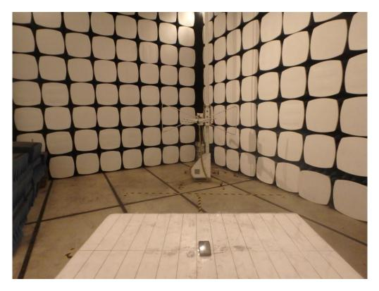
RADIATED EMISSION ABOVE 1G TEST SETUP
