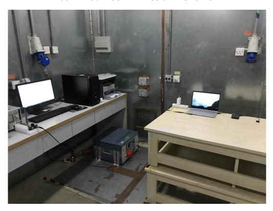
FCC RADIATED EMISSION TEST SETUP
