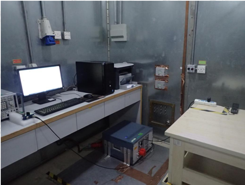
RADIATED EMISSION TEST SETUP
