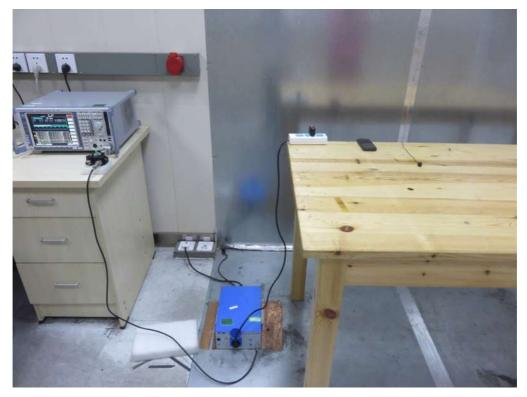
FCC RADIATED EMISSION TEST SETUP
