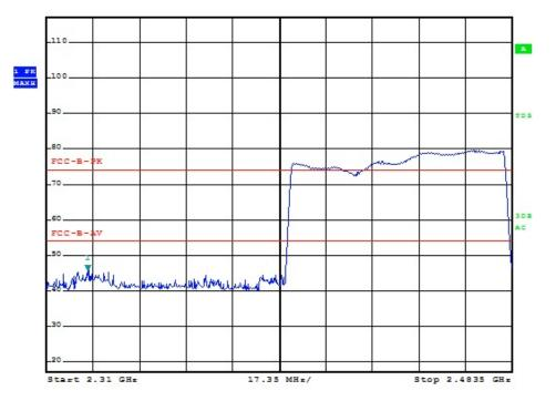
AV Detector: RBW: 1 MHz, VBW: 10 Hz (2 310 MHz - 2 390 MHz), Worst case (Low, Vertical)
