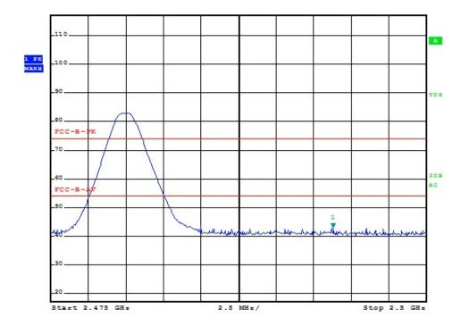
Peak Detector: RBW: 1 MHz, VBW: 1 MHz (2 483.5 MHz - 2 500.0 MHz), Worst case (High, Vertical)
