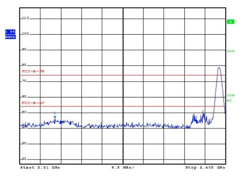
AV Detector: RBW: 1 MHz, VBW: 10 Hz (2 310 MHz - 2 390 MHz), Worst case (Low, Vertical)
