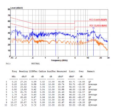
12 13.92 9.11 9.74 0.10 10.00 28.95 50.00 -21.05 Remarks: 1. Measured = Reading + LISNFac + Cable Loss + Aux2 Fac. 2. The emission levels that are 20dB below the official limit are not reported.
