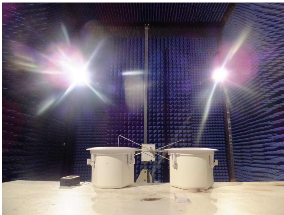
2 Photo of Radiation Emission Test
