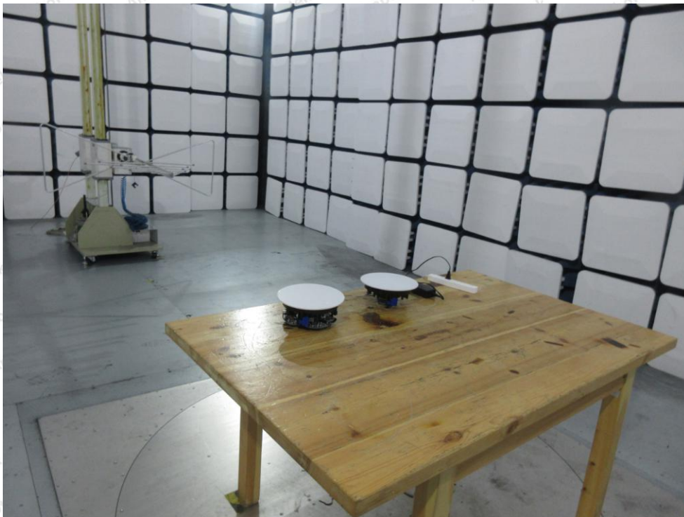
Photo of Radiation Emission Test
