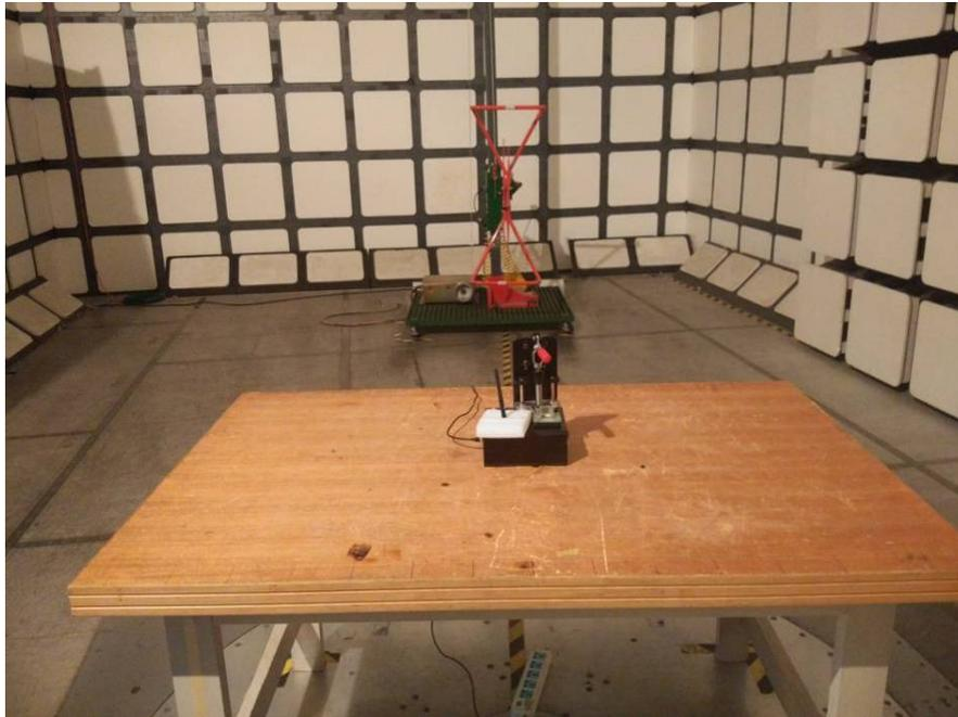
**Radiated Emissions View – External Antenna (Above 1 GHz)**
