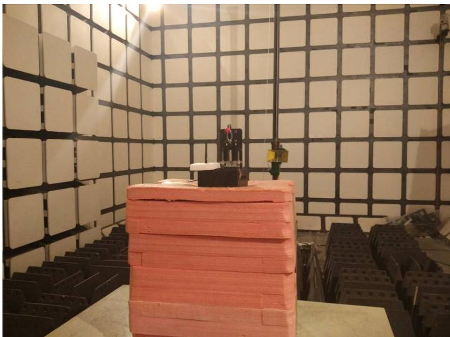
**Radiated Emissions View – Onboard Antenna (Below 1 GHz)**
