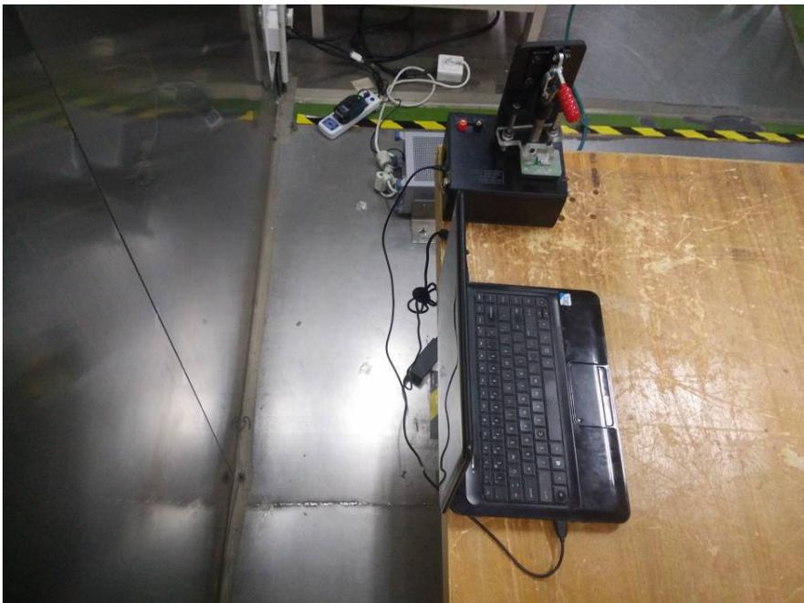
**Radiated Emissions View – External Antenna (Below 1 GHz)**
