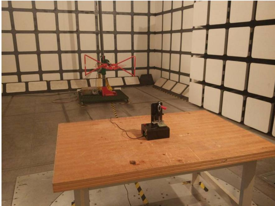
**Radiated Emissions View – Onboard Antenna (Above 1 GHz)**
