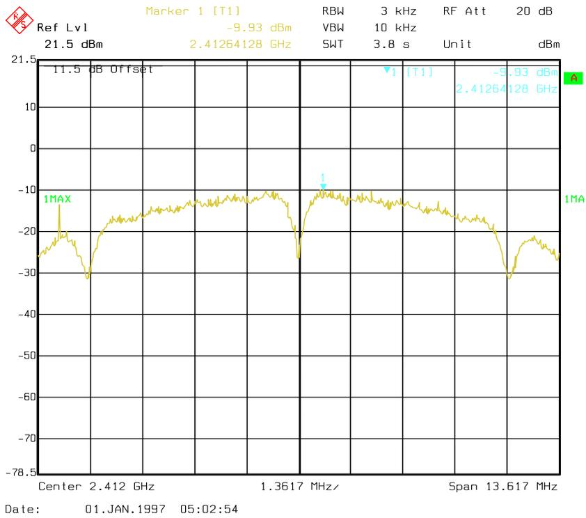
**Power Spectral Density, 802.11b Middle Channel**
