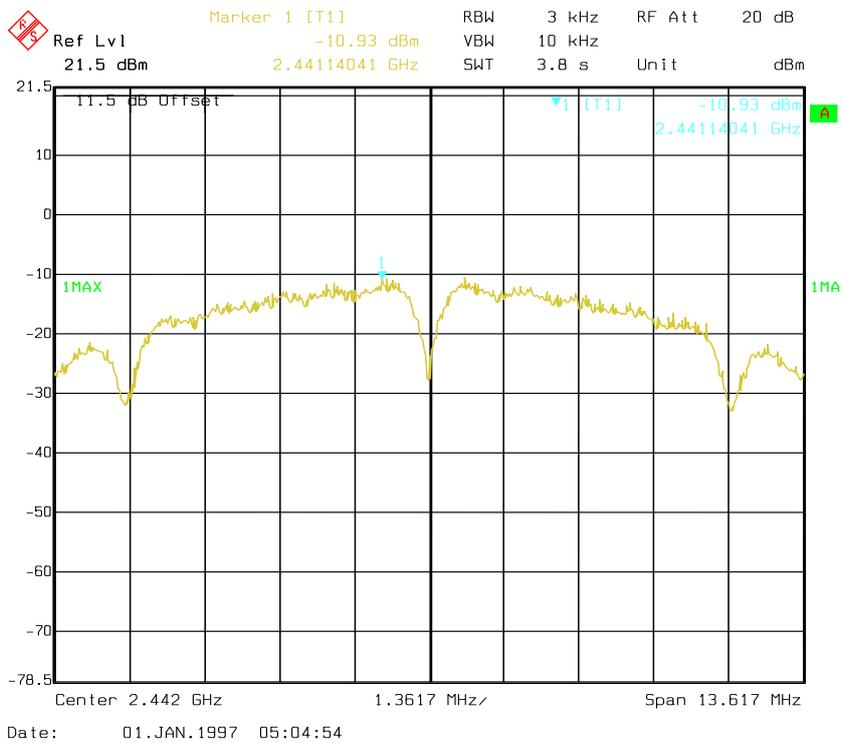
**Power Spectral Density, 802.11b High Channel**
