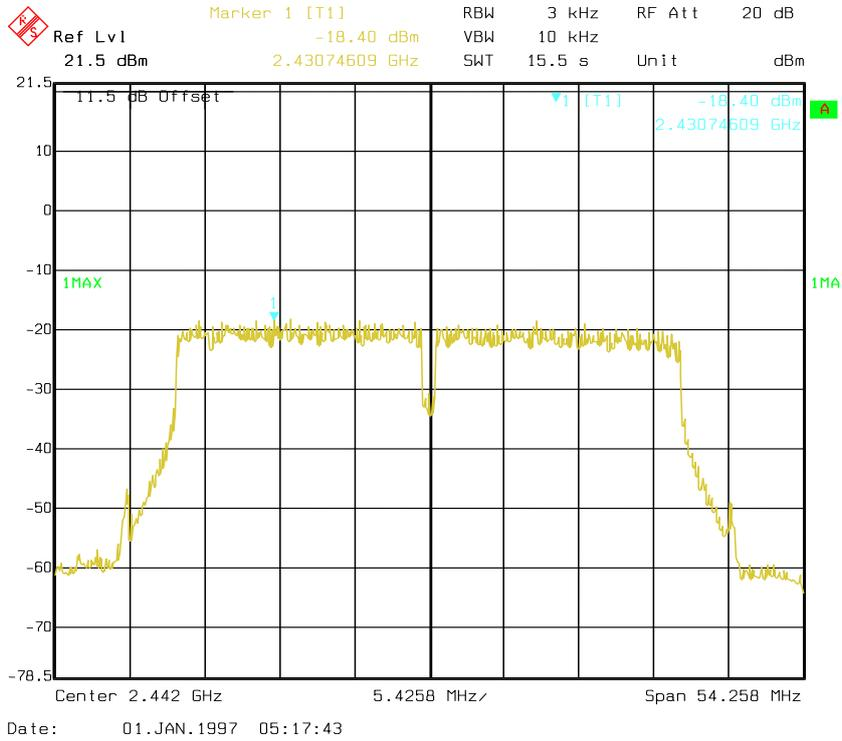
**Power Spectral Density, 802.11n-HT40 High Channel**
