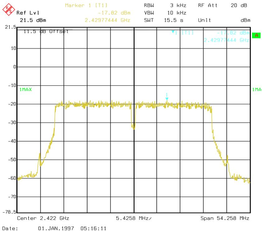
**Power Spectral Density, 802.11n-HT40 Middle Channel**
