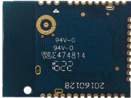
Figure 4-2 RAK476 Bottom View
